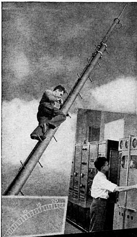
Left: The vertical coaxial antenna, used by W7INY, Frequency Modulation station owned and operated by WOR, New York, is the only one of its kind in existence. It was designed by WOR engineers and is used for FM broadcasting with favorable results.
